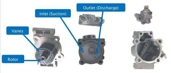
It is important that vane compressors are supplied with oil. Any restriction blocking oil can result in a devastating effect. It is also necessary that the compressor is correctly "primed" before installation. If the compressor is not primed correctly, the vanes will not be lubricated, and upon startup of the air conditioning system, the compressor will not pump correctly. Therefore, the compressor will appear to have failed when it has not.
