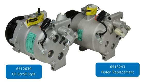
The piston replacement compressor is a direct bolt-off, bolt-on replacement for the OE scroll style design. gpd's piston design is more tolerable of debris left in the A/C system and performs better at lower RPMs than the OE scroll design. Regardless of which compressor is used, gpd highly recommends flushing the system and replacing the condenser.
