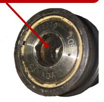
Decoupler pulley must be clean and free of rust/debris.
