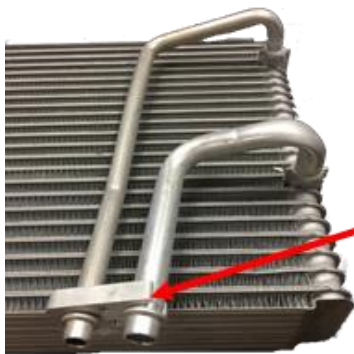
2. Place the clip on the lines of the evaporator (as shown above.)
