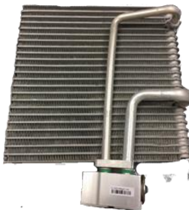
3. Connect the expansion valve to the lines making sure it is turned the proper direction.
