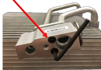
4. Connect the expansion valve to the hardware by using a 4 mm hex to install the screws
