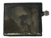
During the process of the heat exchange, the evaporator removes the heat and moisture out of the air inside of the vehicle, which leads to moisture condensation on the outside of the evaporator and evaporator fins. This is more noticeable on a humid day when a puddle of water is formed underneath the car, on the passenger's side. It is originating from the moisture flowing from the face of the evaporator and exiting the vehicle via a drain tube.
