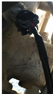
3. Connect the pressure transducer tester between the transducer switch and the electrical connector.
