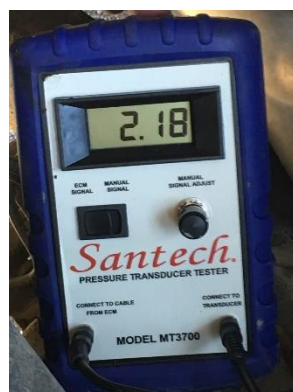
4. As you start the vehicle, the power will engage the tester. This image shows the ECM voltage signal.
