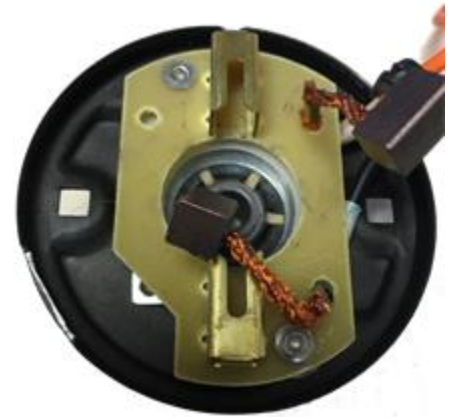
Figure: 1.1: Notice the carbon brushes that can wear over time.
