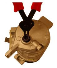
Start by removing snap ring, holding compressor pressure switch in place
