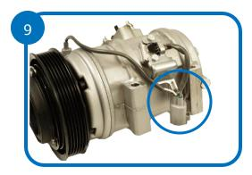
10. Connect switch electrical connector to gpd compressor.
