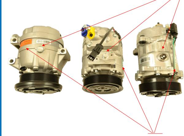
The proper amount of oil for the compressor can be found here on the side of the compressor. Please note that attempting to check the oil level from the manifold connection will not result in a correct measurement. The only way to properly check the oil is to drain the compressor completely through the oil fill bolt as shown above.
