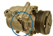
Case damage caused by high pressure from not changing condenser
