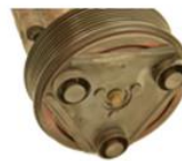
Burnt clutch caused by high pressure or voltage issue
