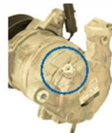
Pop off valve cover missing usually caused by high pressure
