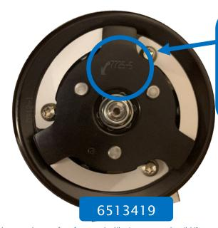
Arrow embedded on clutch to show clutch spins in a counterclockwise direction.
