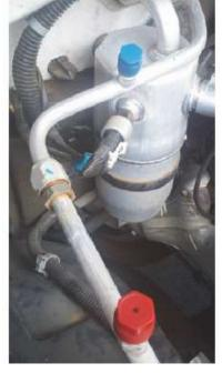
The low side & high side service ports on some GM applications, with the orifice tube in the center.
