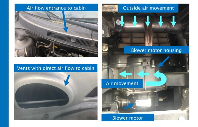
Most late model vehicles use a cabin air filter, typically located above the blower motor housing. Refer to gpd Tech Tip #153, "Precautions to Take When Replacing a Cabin Air Filter".
