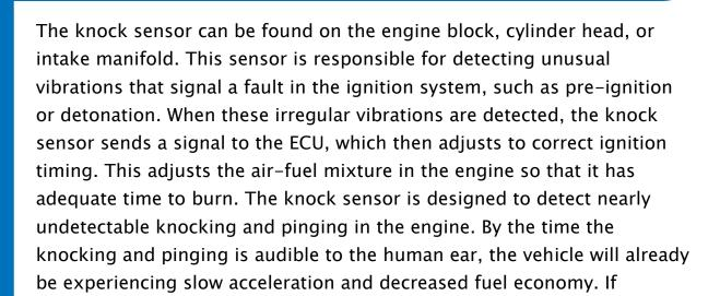
ignored, a faulty knock sensor can damage the engine permanently.
