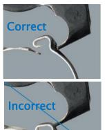
If the pliers are not kept square during closing of the clip, the clasp may have an offset. Use the pliers to correct the clasp alignment. Nose of the pliers should be firmly seated under the assembly bump and lock latch.
