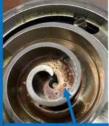
In this image, the water droplets show that moisture has been introduced into the system. This is particularly damaging to hybrid compressors that conduct high voltage electricity.
