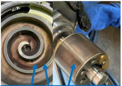
The stationary scroll shown on the left is found in the middle of the compressor and is where refrigerant is discharged. See gpd Tech Tip #54 for an in depth description of scroll compressors. The images above show signs of electrical arcing (dark grey/brown burn marks) due to high pressure and low dielectric properties in the oil.
