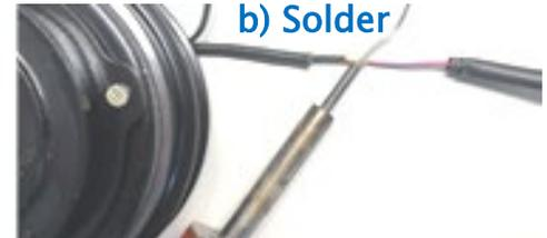
5. Locate the earth strap, the eyelet connection attached to the compressor, where the last earth strap was located. Either tape or heat shrink the connection so it is watertight and cannot short out on another surface
