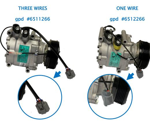
When replacing a compressor, it's good practice to replace the drier, expansion valve, and O-Rings.
