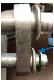
Notice the thin strip of uncovered aluminum. Here a power tool has broken the weld, causing the bracket to shift. The torque of the power tool has also bent the aluminum bracket as one side was tightened first.
