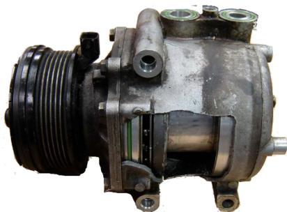
When confronted with a compressor failure on a vehicle fitted with a parallel flow condenser, we recommend that the technician replace the accumulator, orifice tube or expansion device and condenser. We also recommend that all other components are flushed to ensure they are free of contaminants that could harm the new compressor.
