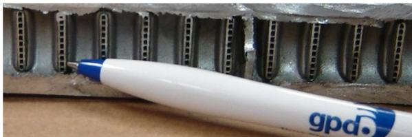
When a compressor fails it introduces contaminants into the system, one of the easiest ways to spot this is to remove the orifice tube that usually reveals metal deposits or sludge from a faulty compressor. The metal and sludge gets deposited throughout the system and will collect at places in the system with restrictions, like the orifice tube and on later model vehicles, the parallel flow condensers.
