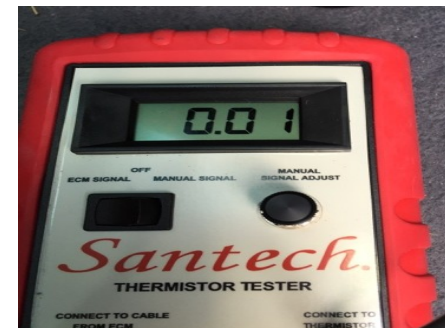
4. Power vehicle on and using the instructions provided, you can measure the resistance coming in from the AC control module or manually control the signal.
