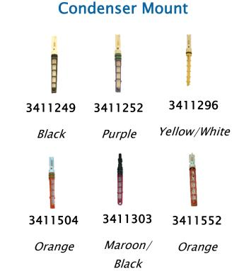
When deciding which orifice tube you should use, remember that color is important. Orifice tube colors identify orifice diameters. Substitution of different color orifice tubes will not work. For example, a white orifice tube cannot be substituted for a yellow or red orifice tube for blue in a Ford. Always follow the manufacturer's recommendations for the exact color and fit.
