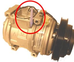
5. Using O-ring pick (gpd# 5811493) remove manifold gasket under shipping plate.
