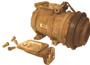
2. Remove 4 x 8mm bolts using caution as compressor may be under pressure. Remove manifold from old compressor taking care not to get any dirt inside manifold. If concerned, clean dirt away.
