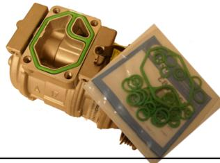
6. If you purchased a gpd compressor kit, it will come with a rapid seal o-ring kit. Locate the manifold gasket and place on compressor where the old one was located.
