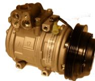
7. Place manifold from old compressor on to your new compressor and tighten. Caution! Note to make sure the manifold is in the right direction, it will fit on the compressor backwards and will have a dramatic effect on the performance of your new compressor. Ensure the manifold is put on the new compressor in the same place/location as when it was taken from the old one.
