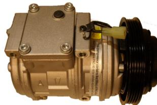
3. Place new compressor facing the same way as the one removed from the vehicle. Locate shipping plate on top of compressor. Undo 4 x 8mm hex bolts. Caution! Every gpd compressor is tested before leaving factory, so there is a high probability that it will be under pressure; use caution when removing plate.
