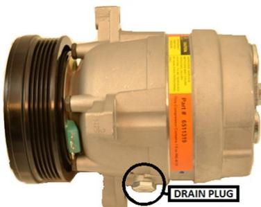
5. Always check the label on the side of the compressor for the correct amount of oil needed in the compressor. Check the oil using the drain plug on the side of the compressor.
