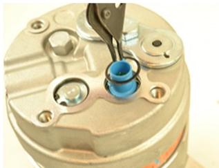
4. Insert snap ring and press around the edges. Ensure that the snap ring seats correctly into the switch port.
