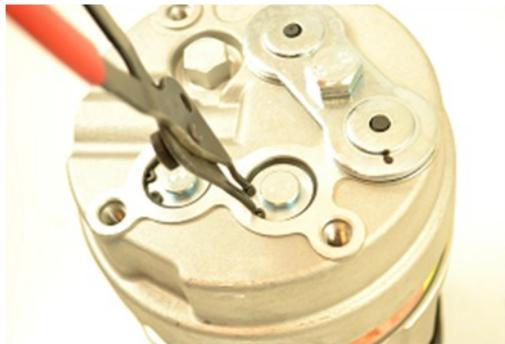
2. Squeeze snap ring that is holding the plug in place.
