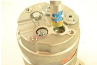
3. Place switch into switch port and press firmly.
