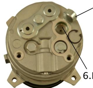
5. Remove & discard Compressor Switch Blank
