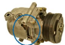
Case damage caused by high pressure from not changing condenser
