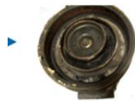
Burnt clutch caused by high pressure or voltage issue
