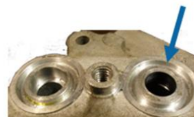
Contamination in suction line shows system contains debris.
