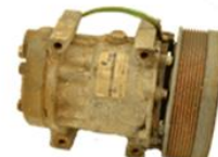
External rust/oxidation usually caused by excessive environmental exposure
