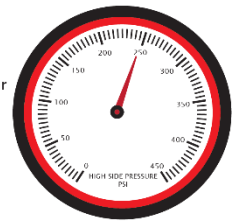
Overcharged or air blocked in the condenser
