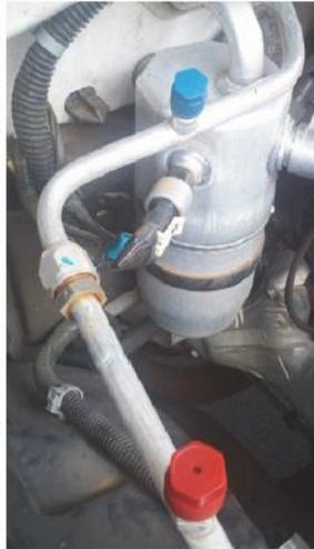
The low side & high side service ports on some GM applications, with the orifice tube in the center.
