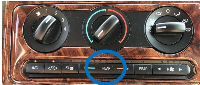
Rear Air Controls
