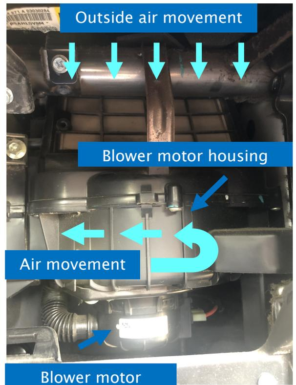
Most late model vehicles use a cabin air filter, typically located above the blower motor housing. Refer to gpd Tech Tip #153, "Precautions to Take When Replacing a Cabin Air Filter".
