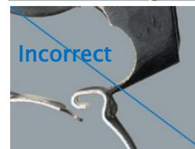
If the pliers are not kept square during closing of the clip, the clasp may have an offset. Use the pliers to correct the clasp alignment. Nose of the pliers should be firmly seated under the assembly bump and lock latch.
