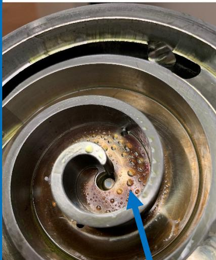
In this image, the water droplets show that moisture has been introduced into the system. This is particularly damaging to hybrid compressors that conduct high voltage electricity.
