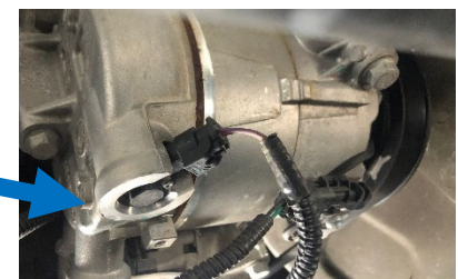
This photo shows the wire connection from the rear of the compressor as it sits in vehicle.
